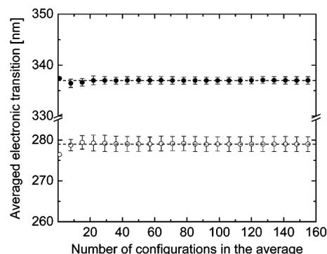
**Figure 6.** Convergence of the calculated transition energies in the absorption spectra of the solvated  $C_{60}$  under ambient conditions. Only the first solvation shell was taken into account in the calculations.
