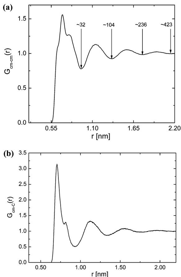
**Figure 2.** Radial distribution functions between  $C_{60}$  and ethanol. (a) In the center-of-mass–center-of-mass RDF, the number of ethanol molecules around the solute is obtained by spherical integration of  $G_{\text{cm-cm}}(r)$ . (b) Profile of the RDF between the center-of-mass of  $C_{60}$  and the carbon atoms on ethanol.
