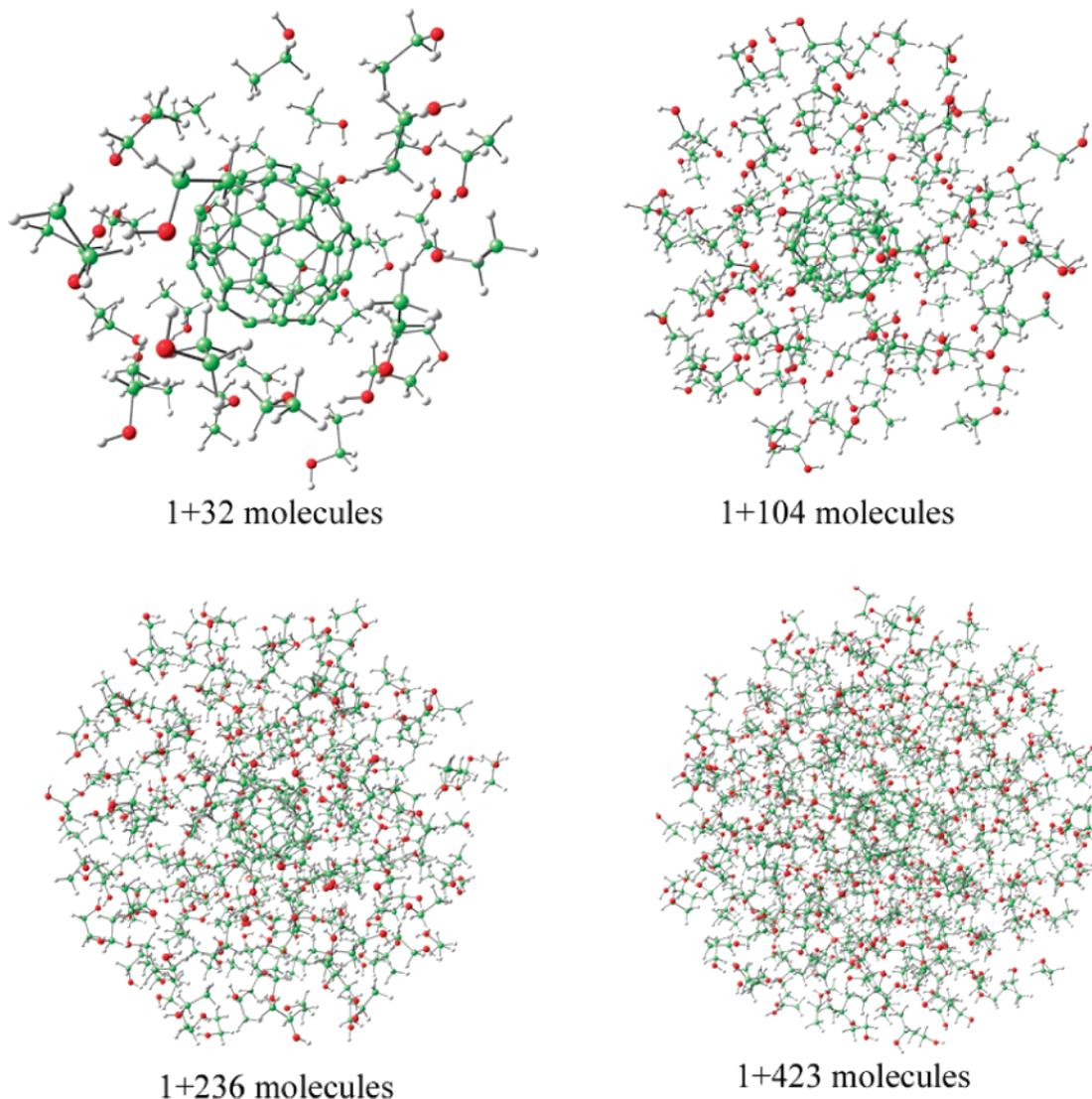
**Figure 3.** Illustration of the structures of the accumulated solvation shells around fullerene in ethanol, as calculated by the RDF spherical integration. Only one single structure of the alcoholic solution is represented.
