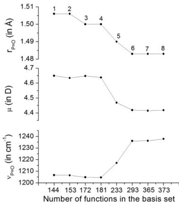
**FIGURE 2.** Convergence of the property with increase of the basis set size. At the top the P=O bond distance in Å, at middle the dipole moment in D and at the bottom the frequency of the  $\nu_{P=O}$  stretching mode in  $\text{cm}^{-1}$ . 1. 6-31+G(d,p); 2. 6-31++G(d,p); 3. 6-311+G(d,p); 4. 6-311++G(d,p); 5. 6-311++G(2d,2p); 6. 6-311++G(3df,2p); 7. 6-311++G(3df,3pd); 8. 6-311++G(3d2f,2p). The relative CPU time from 1 to 8 is 1/1.3/1.8/3.0/13.5/16.8/28.7/33.4.
